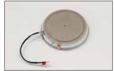
Injection Enhanced Insulated Gate Transistor (IEGT). Rated 4,500 Volts, 2,100 Amps
